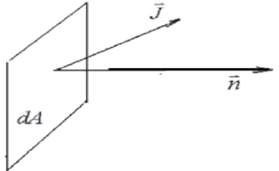
$$J = -\frac{\lambda_s}{3} \left[ \frac{\partial \varphi(r)}{\partial x} \cos \alpha + \frac{\partial \varphi(r)}{\partial y} \cos \beta + \frac{\partial \varphi(r)}{\partial z} \cos \gamma \right]$$
